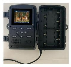
3. Insert the Micro SD card (4GB -128GB) with the chip side down.
