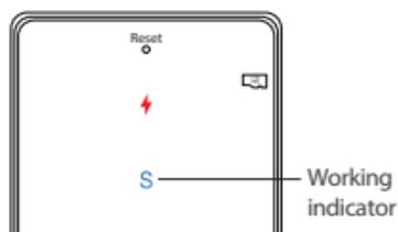
3.A, Long press ON/OFF for 2 seconds, the blue working indicator "S" is on means the device is on. And release the button and the indicator will be off.
