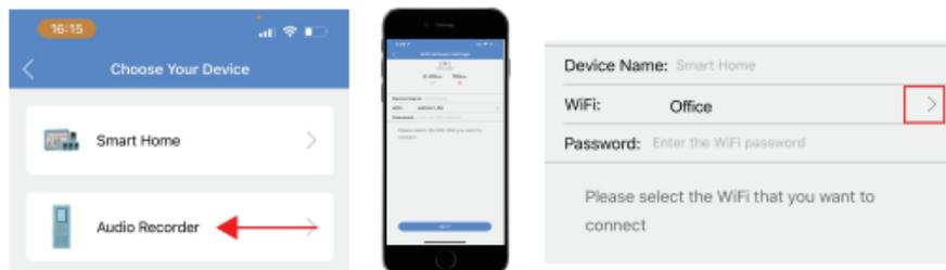
4. Open APP CamSC Pro >> Click + >> Audio Recorder >> Device in pairing mode >> CAM-xxxxxx >> Select 2.4G Wi-Fi >> Input password >> NEXT.
